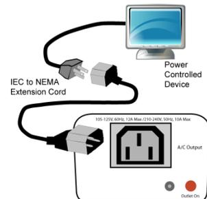
Fig. 2 Connect Device
