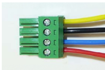
Proper Screw Terminal Connections
